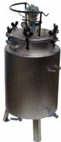
CP-33 80L SS electroplated Dual-layered Pressure Tank with 1/4hp air motor
