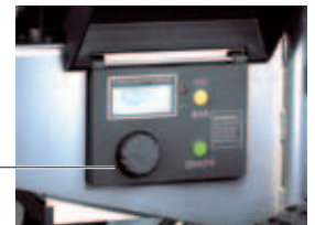
Quick-response electronic pressure control with LCD screen. * BAR or PSI LCD screen available
